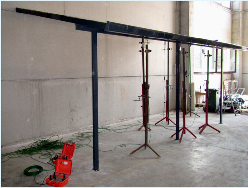
Photos of veranda showing displacement transducer arrangement on the underside
