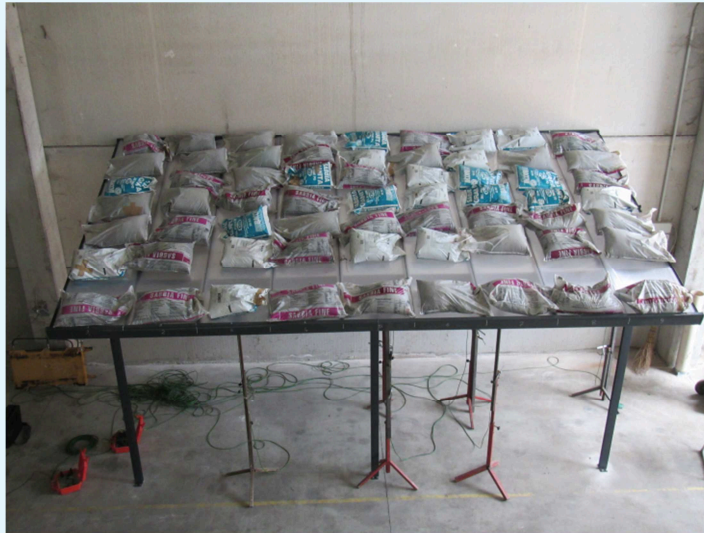
Photo of veranda showing sandbag distribution during load step 3
