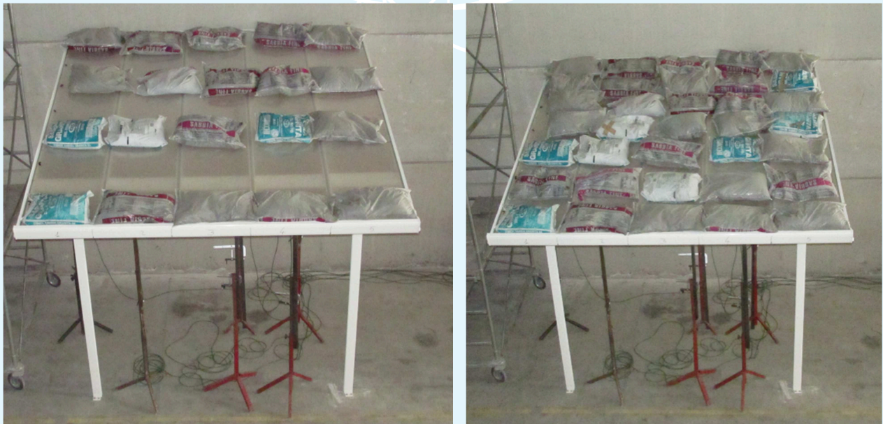
Photos of veranda showing sandbag distribution during load steps 2 and 3
