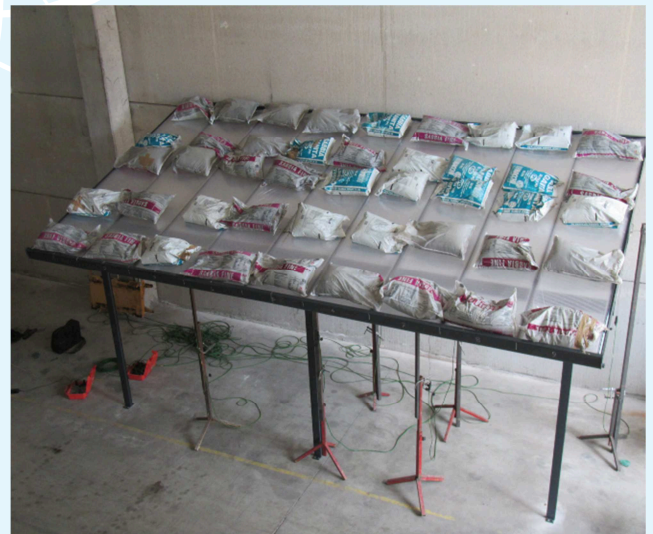
Photos of veranda showing sandbag distribution during load steps 1 and 2
