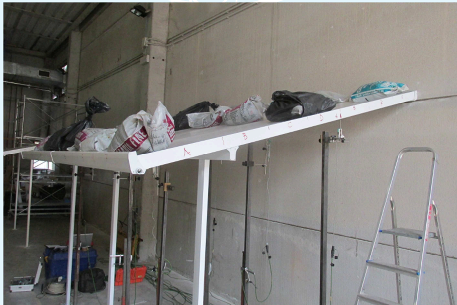
Photo of veranda showing sandbag distribution during load step 1
