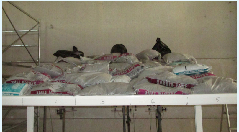
Photos of veranda showing sandbag distribution during maximum load step 5
