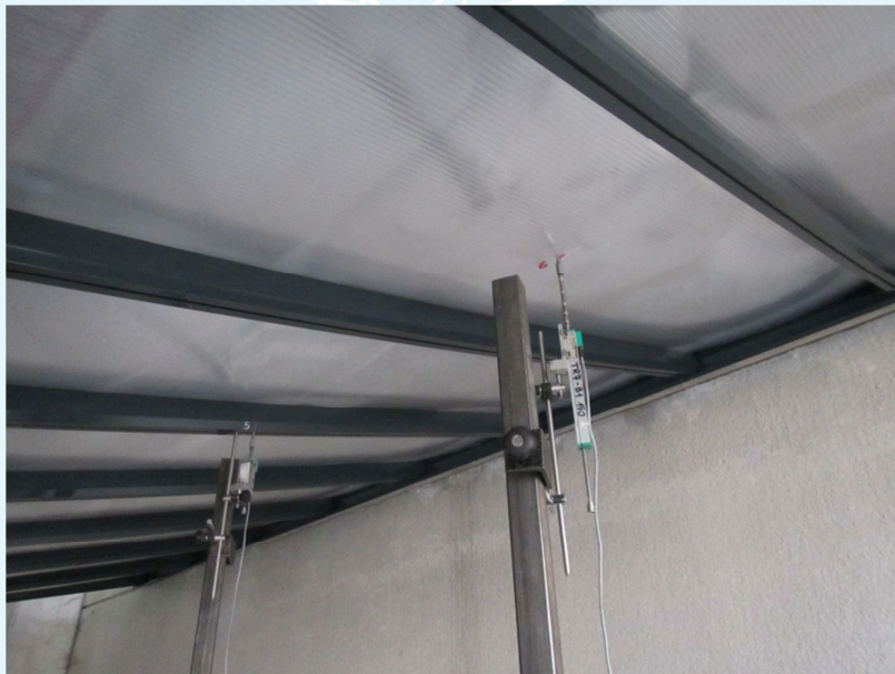
Photo of veranda showing polycarbonate sheets during maximum load step 5
