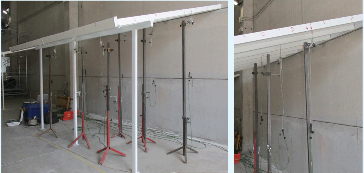
Photos of veranda showing displacement transducer arrangement on the underside
