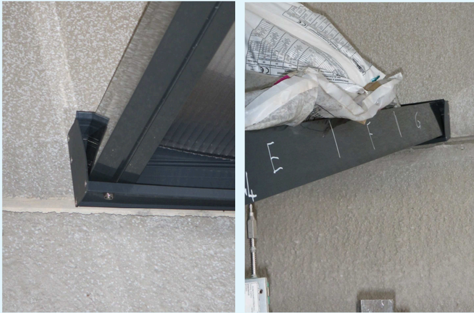
Photos of veranda showing end sections during maximum load step 5
