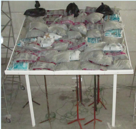
Photos of veranda showing sandbag distribution during maximum load step 5
