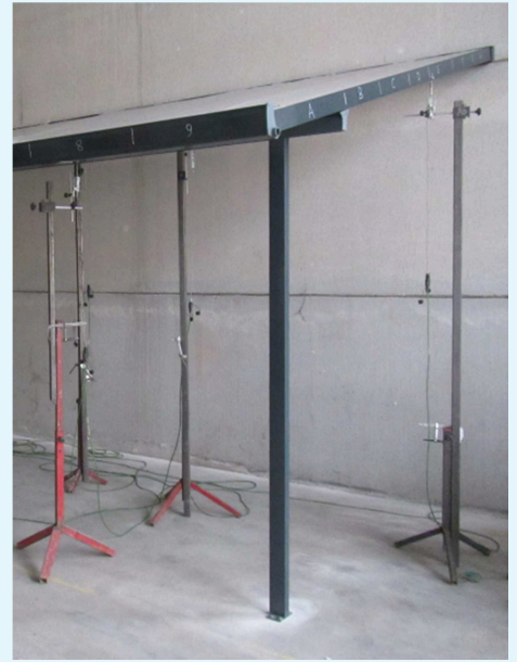
Photos of veranda showing displacement transducer arrangement on the underside
