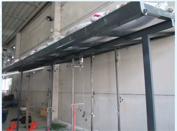
Photos of veranda showing sandbag distribution during maximum load step 5
