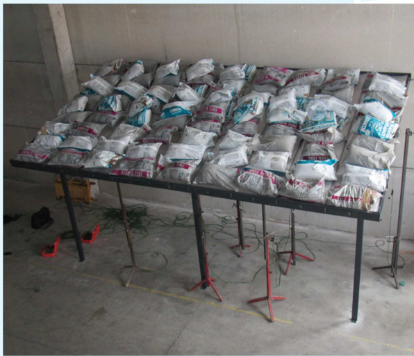
Photos of veranda showing sandbag distribution during maximum load step 5
