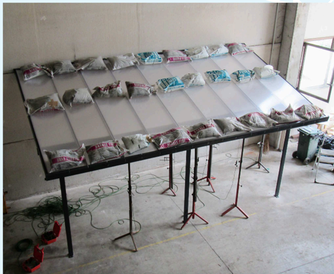
Photos of veranda showing sandbag distribution during load steps 1 and 2
